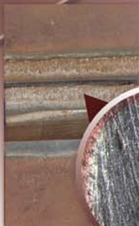
Fracture of weld seam with SigmaWeld 199
