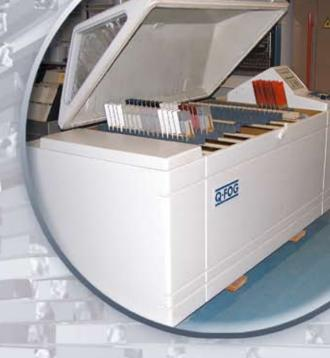
A humidity cabinet is used for accelerated testing to evaluate the coatings resistance in very humid environments
